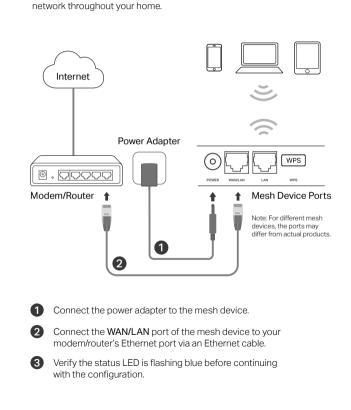
The Whole Home Mesh Wi-Fi AP is designed to create a mesh wireless
